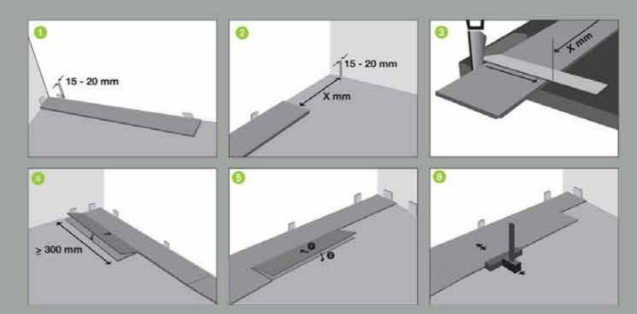
Step1. The B plate tenon plate A inclined in the fillster locking, and then put it flat.
